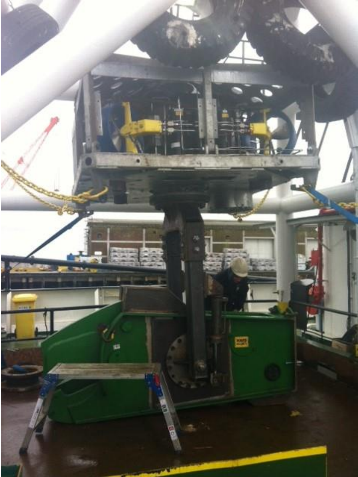
Shear grab fitted to the ROGE for the 1 st time, the tilt frame allows for the shear to be adjusted between the horizontal and vertical position
